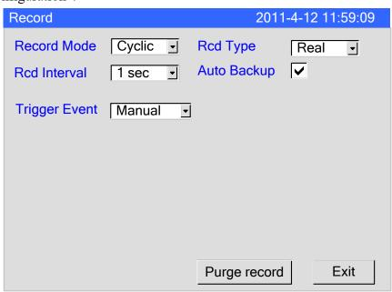
Recording: This column is used to set recording method.
