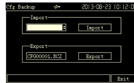
Configuration backup Free input and output of configuration information, easy configuration setting.
